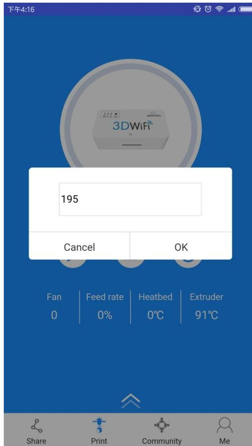
Step 2. Click [Heat up] button
